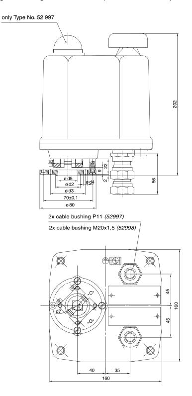
Connecting dimensions for actuator connection to a valve (any other connection should be consulted with the manufacturer beforehand).
