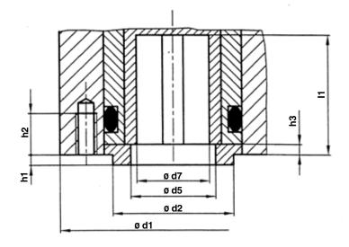
The position of groove for keyway according to ISO 5211 and DIN 3337 is in the position "Closed". The position "Opened" is to the left of the position "Closed" when viewing in the direction to the local indicator of position. The position "Z" ("C") of the groove for keyway is identical with the position "Z" ("C") on the local indicator of position.
