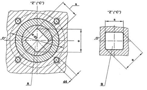
A – connection by square in basic position B – connection by square turned by 45  $^\circ$
