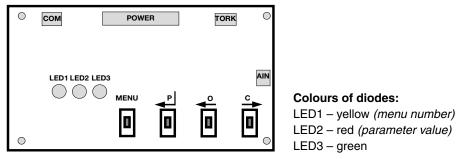
Push-buttons and signal lamps LED on control unit DMS2.ED.S and DMS2.ED.S90
