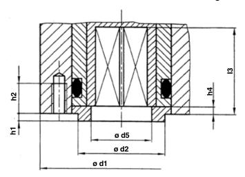
The position of the square hole in end position of electric actuator. The position "Opened" is to the left of the position "Closed" when viewing in the direction to the local indicator of position. The square hole is according to DIN 79:2013-02. Connecting dimensions are according to DIN 3337 or ISO 5211. The position "Z" ("C") of the square hole for spindle
