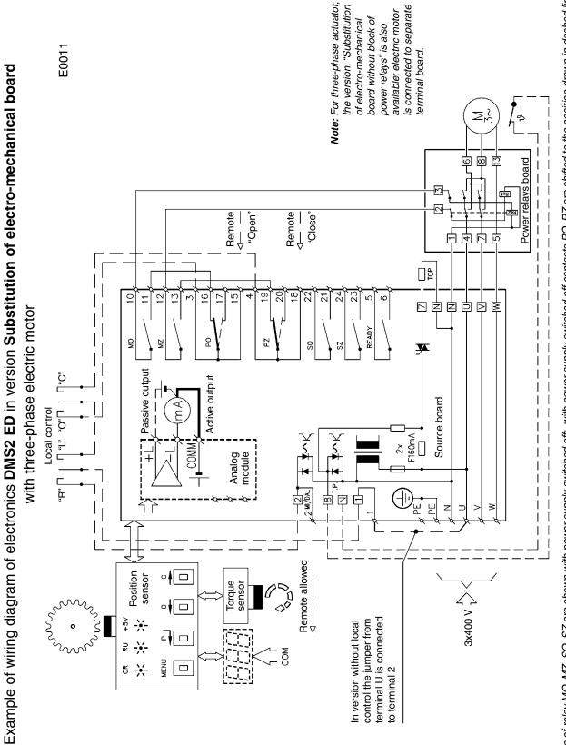
Note: Here, contacts of relay MO, MZ, SO, SZ are shown with power supply switched off; with power supply switched off contacts PO, PZ are shifted to the position drawn in dashed line.
