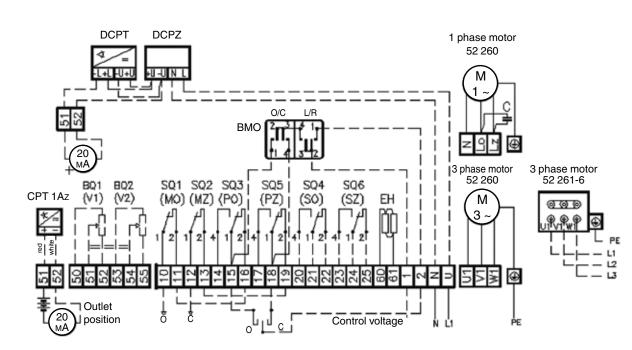
Wiring diagram of electric actuators MODACT MPS, MPSP Control - with contactors
