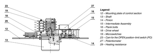
Fig. 6b - Connection of resistive transmitter with drive in actuators 52 261-52 266
