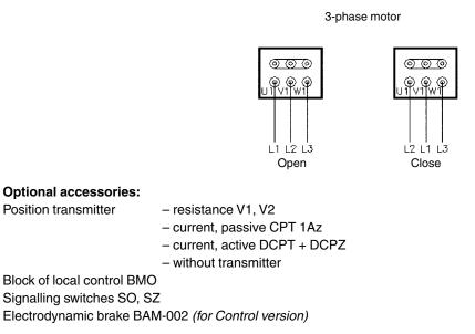
Note: The actuators MODACT, MPS, MPSP 52 261-6 with resistance transmitter V1, V2 are not fitted with the signalling switches SO, SZ.
