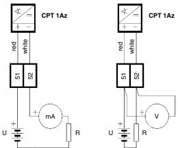
4. Use a voltmeter to check the voltage on the CPT 1Az terminals. In order to keep linearity of the output signal the voltage must not drop below 9 V, not even with off-take 20 mA. If this condition is not met it is necessary to increase the feeding voltage (within the range of recommend values) or to decrease total resistance of the current loop R.
