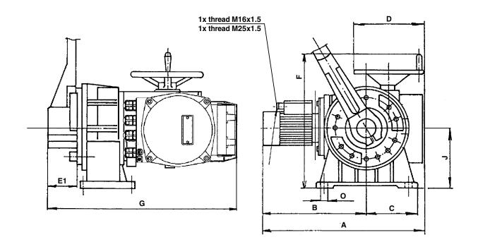
**Note:** Threads for cable bushings in the terminal box: 1 x M25 x 1.5, 3 x M20 x 1.5 (cable bushings are included – attached).
