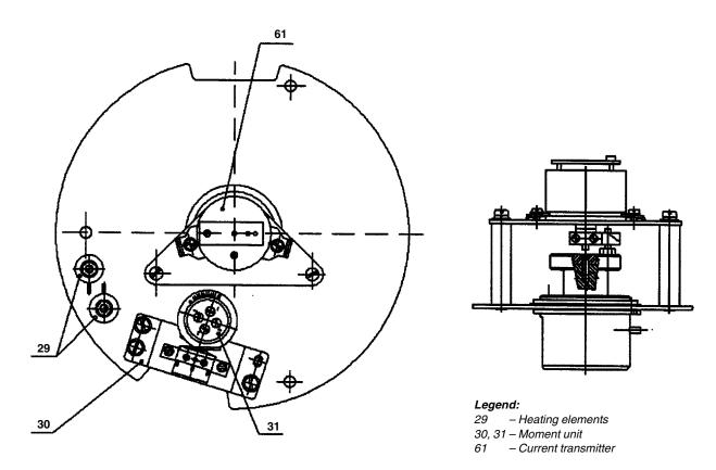
Fig. 4 – **Base plate with current transmitter** – without position and signalling switches – transmitter directly on output shaft (this version is designated with the digit 9 at the second place of the supplementary number, e.g. 52 261.x9xx)
