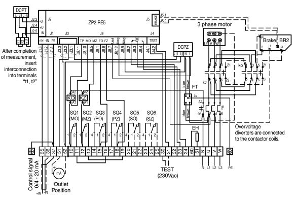
Wiring diagram of electric actuators **MODACT MPS**, **MPSP Control**, **T. No. 52 261- 6** – with BMO and regulator ZP2.RE5
