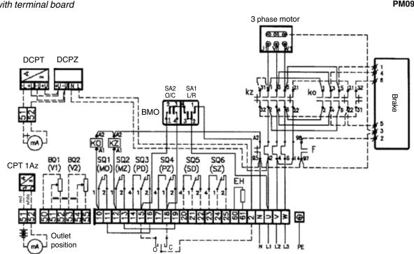
Wiring diagram of electric actuators MODACT MPS, MPSP Control, T. No. 52 261-6, - with regulator ZP2.RE5
