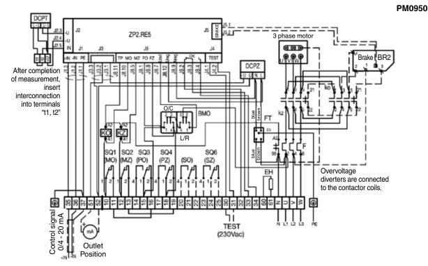
Wiring diagram of electric actuators MODACT MPS, MPSP T. No. 52 260 and 52 261-6
