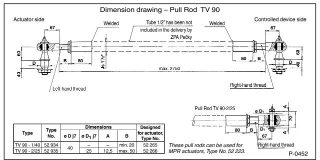
Designed for connecting the actuators to the controlled device, these pull rods provide for the transmission of movements of the output section of the actuators to the controlled device. Not included in the delivery, they should be ordered separately.
