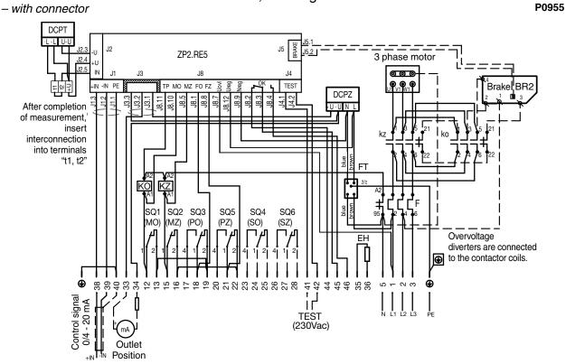
Wiring diagram of electric actuators **MODACT MPS**, **MPSP Control**, **T. No. 52 261-6**, – with contactors, with BMO and regulator ZP2.RE5
