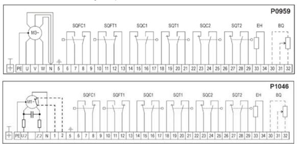
Design with potentiometer or without transmitter
