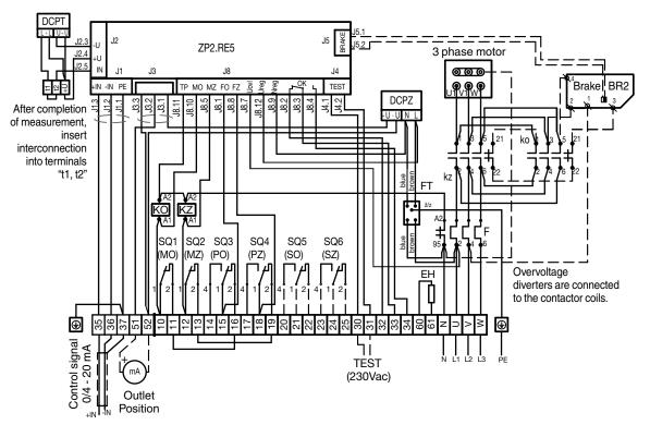
Wiring diagram of electric actuators **MODACT MPS, MPSP Control, T. No. 52 261-6** – with BMO and regulator ZP2.RE5
