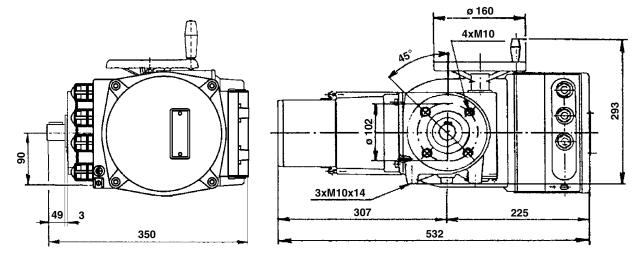
**Note:** Threads for cable bushings in the terminal box: 1 x M25 x 1.5, 3 x M20 x 1.5 (cable bushings are included – attached).
