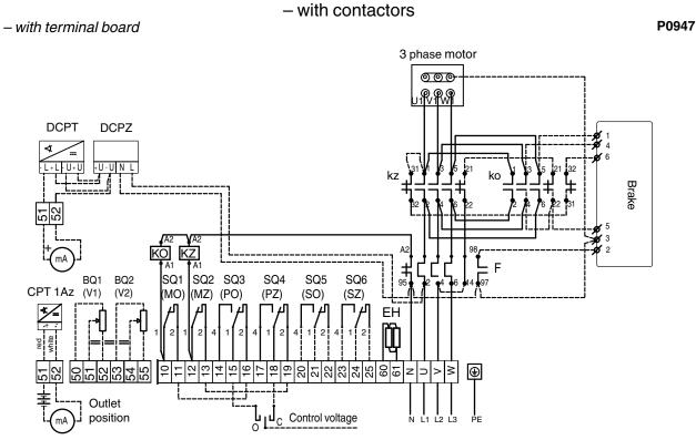
Wiring diagram of electric actuators **MODACT MPS Control** – with contactors and BMO
