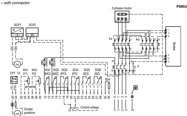
Wiring diagram of electric actuators **MODACT MPS, MPSP Control** – with contactors and BMO
