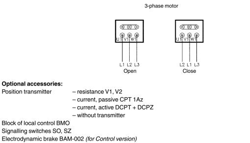
Note: The actuators MODACT, MPS, MPSP 52 261-6 with resistance transmitter V1, V2 are not fitted with the signalling switches SO, SZ.
