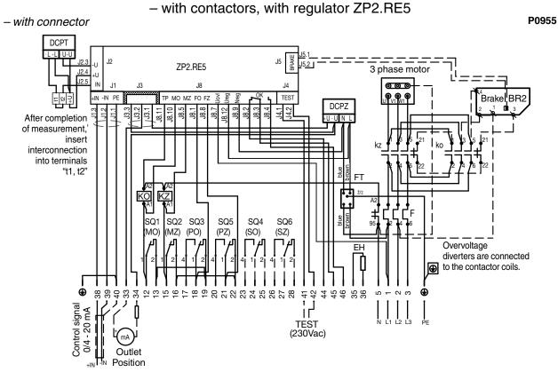
Wiring diagram of electric actuators **MODACT MPS, MPSP Control, T. No. 52 261-6,** – with contactors, with BMO and regulator ZP2.RE5
