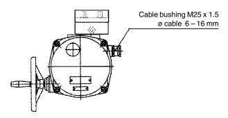
Mechanical connecting dimensions of **MODACT MOPED** electric actuator, type no. 52 039
