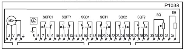
Position transmitter - current 4 - 20 mA or without transmitter
