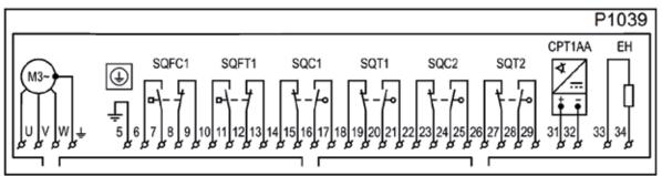
Position transmitter - current 4 - 20 mA with feeding source
