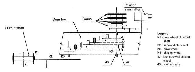
Fig. 5 - Kinematic diagram of gearings
