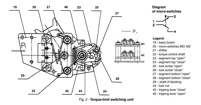
The numbers on this scale do not show setting of tripping torque directly. Divisions on this scale serve just for more precise dividing of the range of points of maximum and minimum tripping torque and, thus, more precise resetting of tripping torque out of the factory in case a loading bench is not at disposal. Segment 28 is intended for direction "close", segment 27 for direction "open".
