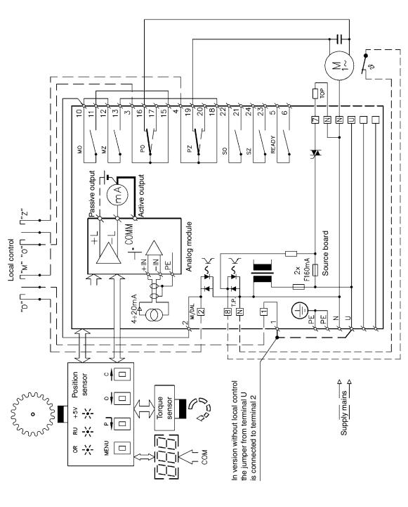
Note: Here, contacts of relays MO, MZ, SO, SZ are shown with power supply switched off; with power supply switched off contacts PO, PZ are shifted to the position drawn in dashed line.
